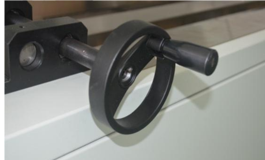
Board width Adjustment Handle Adjust wide:0-300MM
